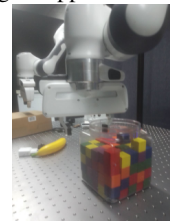
Fig. 10: Experiment setup of the circular object grasping task.
